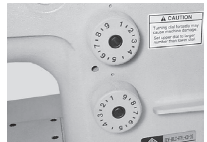
One touch switchover for two different stitch lengths (DS device)
