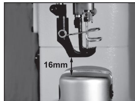
The clearance under the presser foot (16mm)
