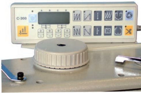
Simple setting for walking foot movement
