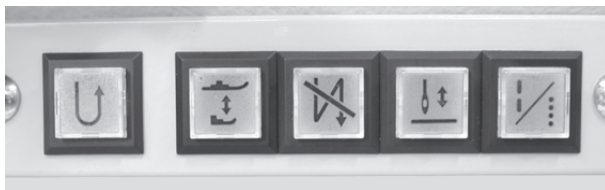
Simple setting for walking foot movement
