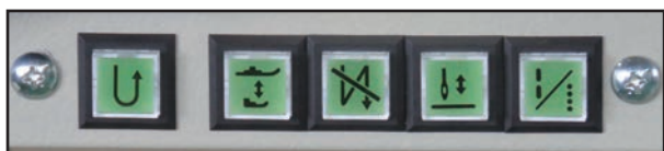
Simple setting for alternating presser foot movement
