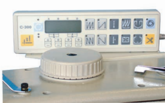
Simple setting for walking foot movement
