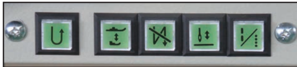
Simple setting for alternating presser foot movement
