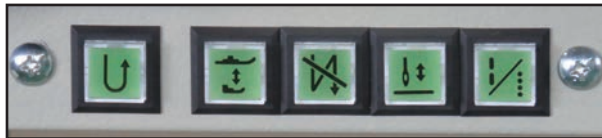
Simple setting for alternating presser foot movement
