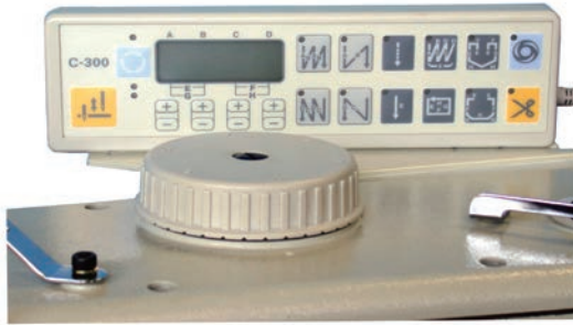
Simple setting for alternating presser foot movement
