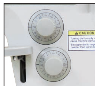
One touch switchover for two different stitch lengths(Dual stitching device)
